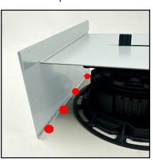
**Step 6:** Allow for Ardex CA20P Adhesive Silicone Spot Bonding at base of profile edge to perimeter flashing.
