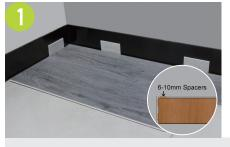
• Provide a 10mm expansion gap between the Max Floor and your walls or fixed objects. This is allowance for the minimal expansion rate which is -/+ 0.1% average. When skirting is installed, ensure there is an expansion gap beneath.
