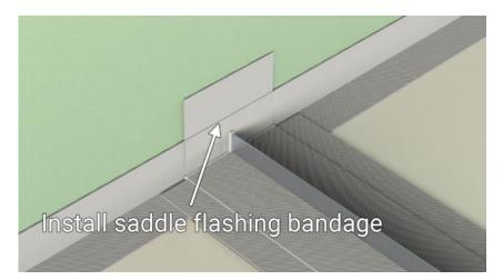
Once the self adhesive buytl tape has been installed either side of the NT Waterstop, a saddle flashing is to be applied over the termination point to aid in sealing the NT Waterstop.
