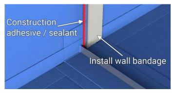
After installing the NT Wall Waterstop measure and cut the self-adhesive butyl tape to the same length as the NT Wall Waterstop.
