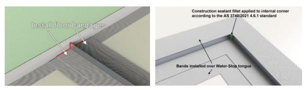
Once the NT Waterstop has been installed correctly, the self adhesive butyl tape can be applied
