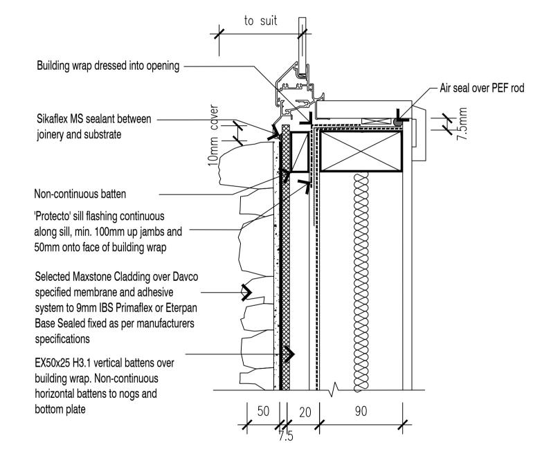
**NOTE:** EX50X25 BATTENS CAN BE SUBSTITUTED WITH EX50X50 WHERE APPROPRIATE
