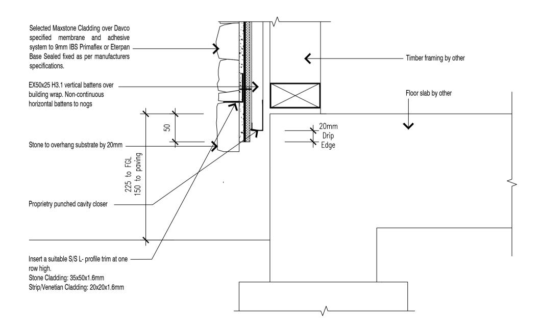
**NOTE:** EX50X25 BATTENS CAN BE SUBSTITUTED WITH EX50X50 WHERE APPROPRIATE
