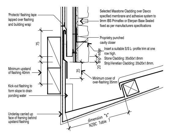
NOTE: EX50X25 BATTENS CAN BE SUBSTITUTED WITH EX50X50 WHERE APPROPRIATE
