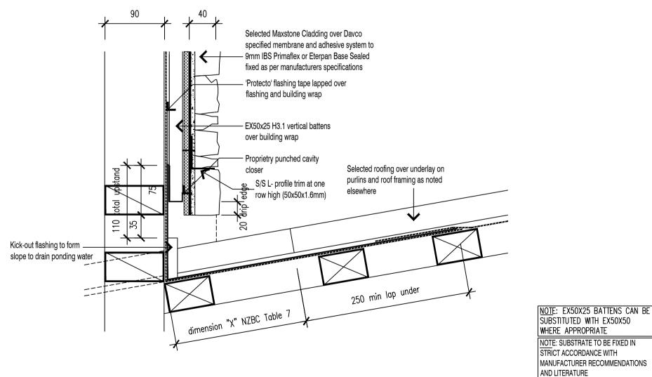
ROOF ABUTMENT DETAIL LONGRUN ROOFING
