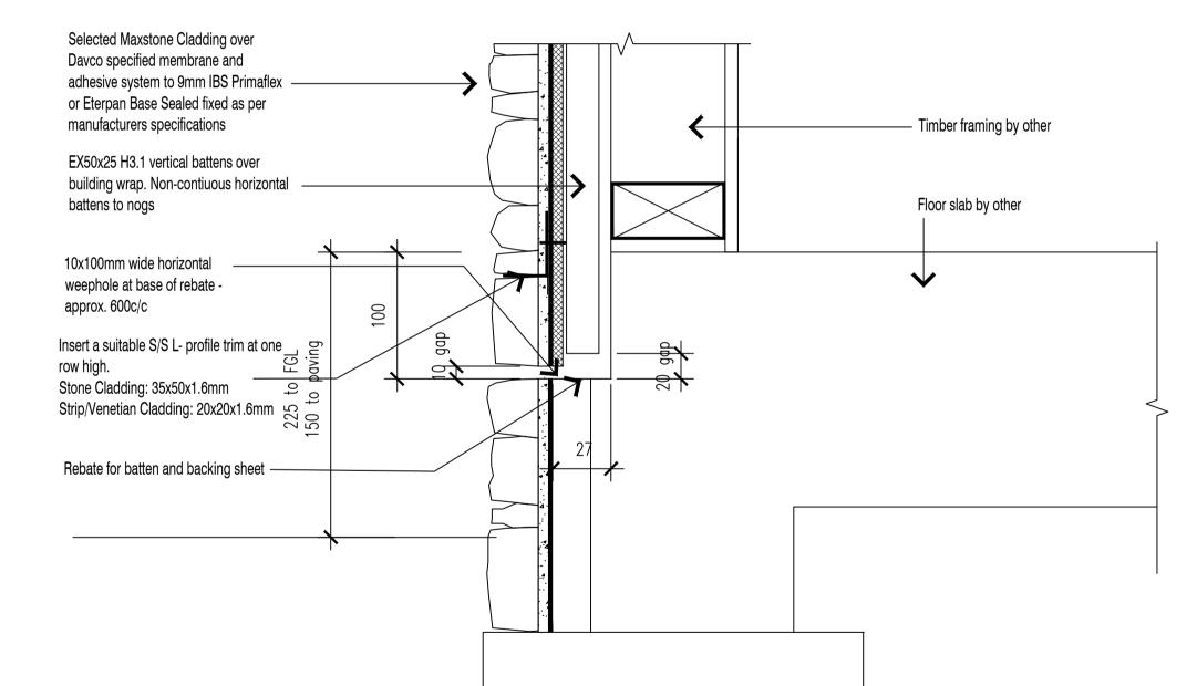
**NOTE:** EX50X25 BATTENS CAN BE SUBSTITUTED WITH EX50X50 WHERE APPROPRIATE
