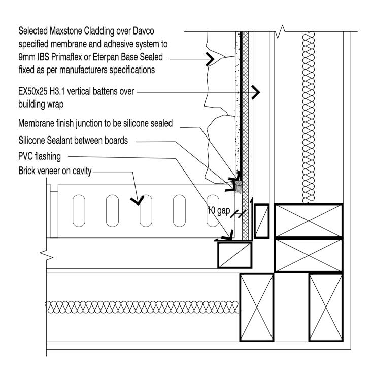
NOTE: MEMBRANE FINISH JUNCTION TO BE SILICONE SEALED
