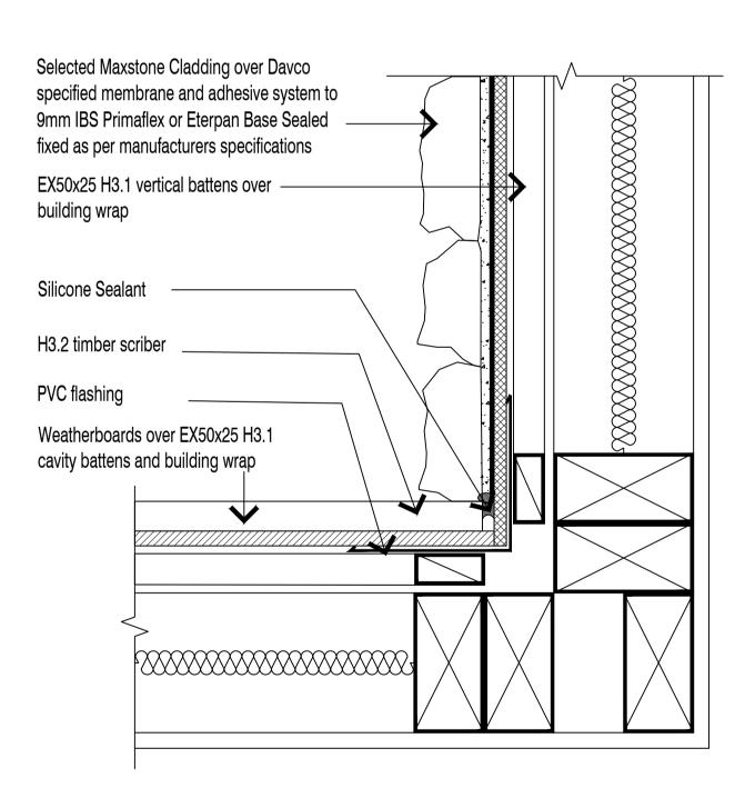
NOTE: MEMBRANE FINISH JUNCTION TO BE SILICONE SEALED
