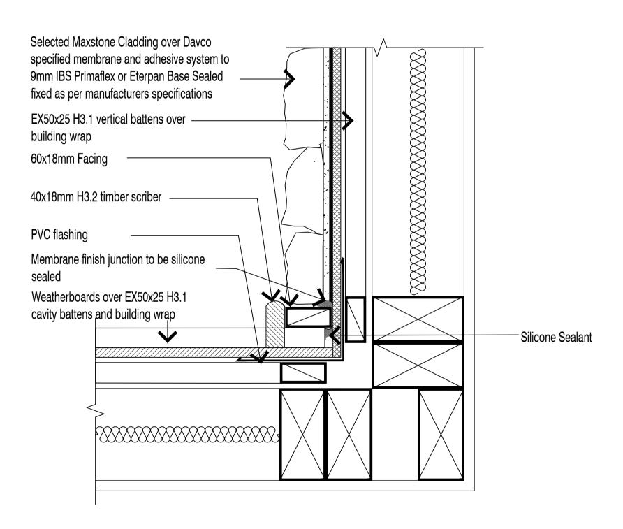
NOTE: MEMBRANE FINISH JUNCTION TO BE SILICONE SEALED
