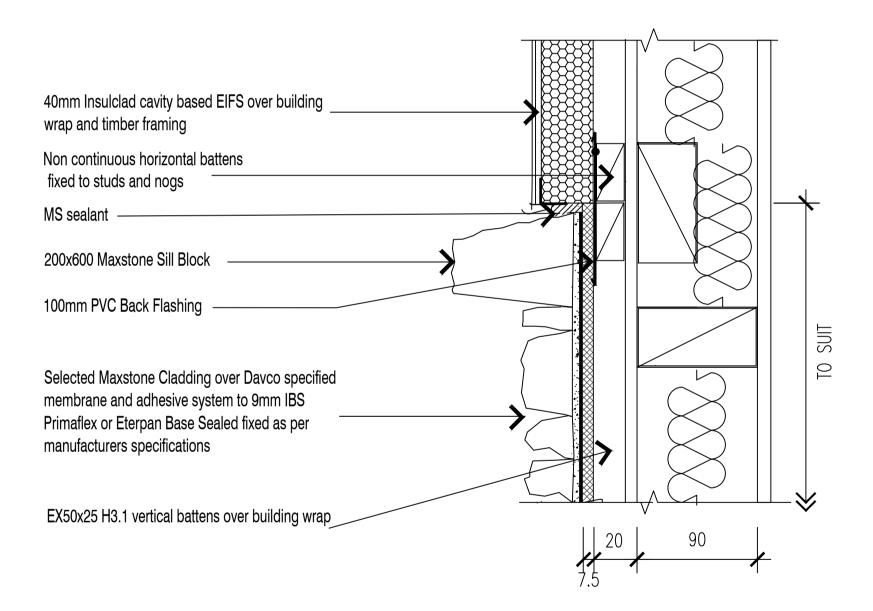
**NOTE:** EX50X25 BATTENS CAN BE SUBSTITUTED WITH EX50X50 WHERE APPROPRIATE
