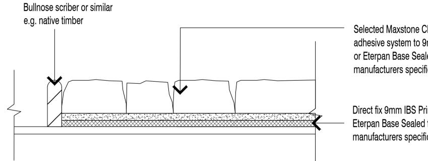
Selected Maxstone Cladding over Davco adhesive system to 9mm IBS Primaflex or Eterpan Base Sealed fixed as per manufacturers specifications
