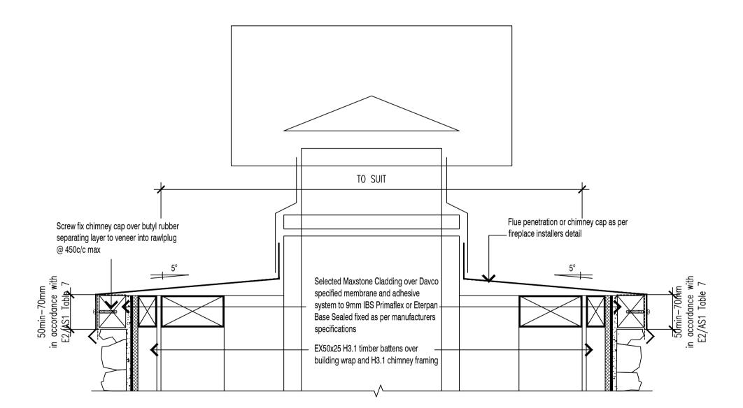
**NOTE:** EX50X25 BATTENS CAN BE SUBSTITUTED WITH EX50X50 WHERE APPROPRIATE
