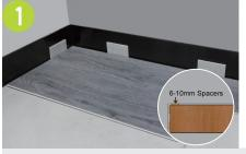
• Provide a 6mm - 10mm expansion gap between the Max Floor and your walls or fixed objects. This is allowance for the minimal expansion rate which is -/+ 0.1% average.
