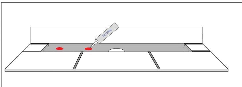
**c)** Lower the channel insert in onto the dabs of adhesive and leave it to cure before proceeding further.
