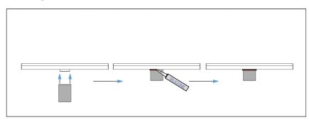
**b)** Apply dobs of neutral cure silicone or a solvent free polystyrene friendly construction adhesive such as Sikaflex®-123 MS Bond.
