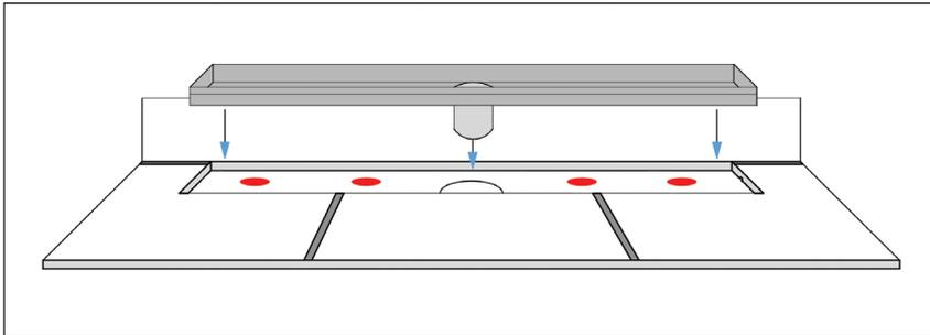
**d)** Seal around the perimeter between the channel drain and the wall and the channel drain and the shower base (where the tiles meet) with a neutral cure silicone and allow to cure.
