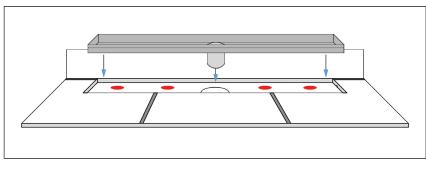
**d)** Seal around the perimeter between the channel drain and the wall and the channel drain and the shower base (where the tiles meet) with a neutral cure silicone and allow to cure.
