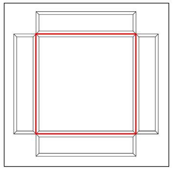
**b)** Fold each of the 4 edges up to create a box and tape the outside of each corner to allow the silicone to cure in place
