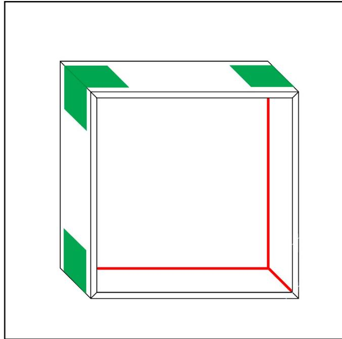
**d)** Zigzag a bead of construction adhesive (as above) onto the wall framing and then insert the niche into the gap.
