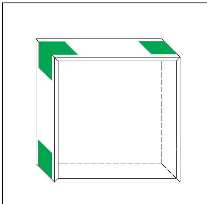
**c)** Run a bead of construction adhesive (Use a solvent free polystyrene friendly construction adhesive such as Sikaflex®-123 MS Bond). along each of the inside corners and allow to cure.
