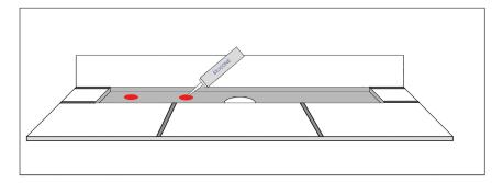
**b)** Lower the channel insert in onto the dabs of adhesive and leave it to cure before proceeding further.
